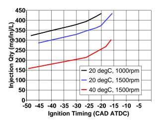
Figure 7. Injection quantity versus ignition timing required for ambient starting of the engine operating with M100.
