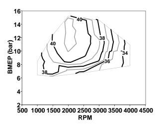
Figure 3. Brake thermal efficiency as a function of engine load and speed for E100 (no denaturant).
