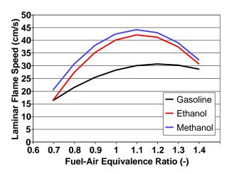
Figure 1. Laminar flame speed of M100, E100 and gasoline as a function of fuel-air equivalence ratio (1 atm, 300K).
