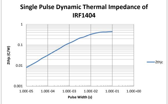
Figure 4 - Zthjc of the IRF1404 Planar MOSFET
