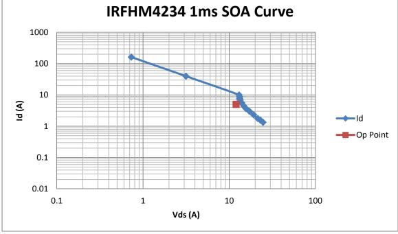
Figure 7 - IRFHM4234 1ms SOA compared to operating point
