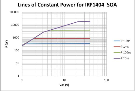
Figure 3 - Constant Power lines of the SOA for the IRF1404 (Planar MOSFET)
