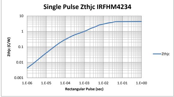
Figure 8 - IRFHM4234 Single Pulse Thermal Impedance Curve
