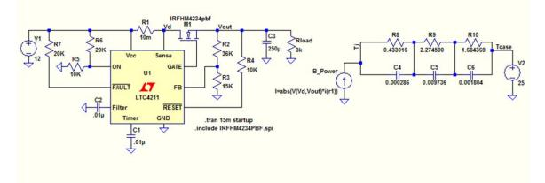
Figure 9 - Hot Swap Simulation Schematic
