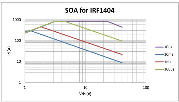
Planar MOSFETs have a SOA that are a family of parallel lines plotted on a log-log graph.
