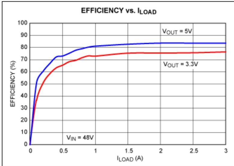
Figure 3. Efficiency vs. load current for the circuit in Figure 1.
