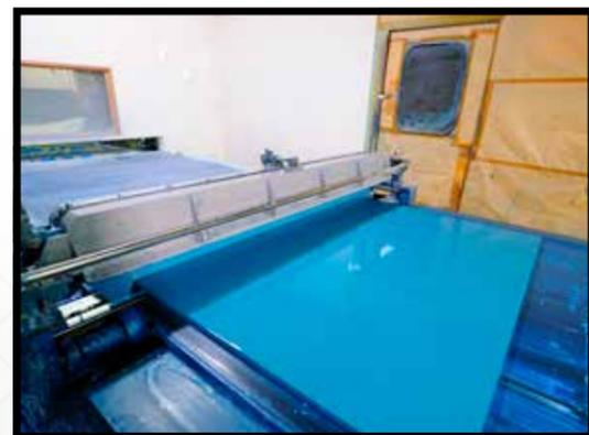
Underneath a veritable waterfall of paint, tabletops pass by at high speed as the thick, uniform coats are completed.
