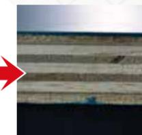
Multiple layers are clearly seen in this cross-section of the finished tabletop.
