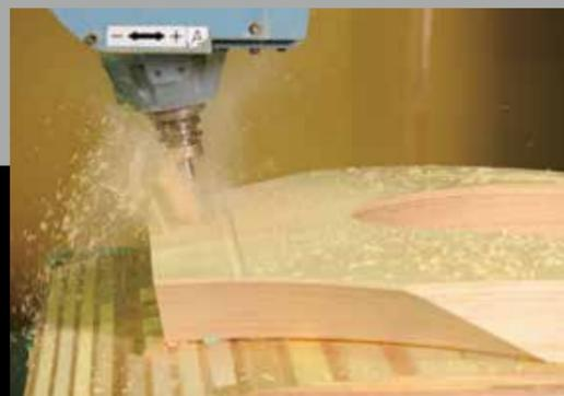
A mass of laminated wood, looking exactly like baumkuchen, is scraped down in this process.
