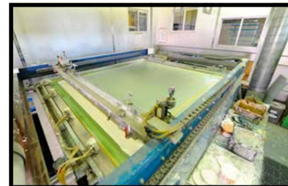
The process of printing the white line on the tabletop surface.
