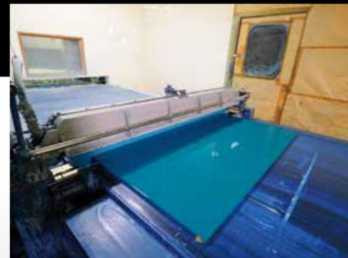
The "les yeux bleus" paint is applied in a curtain-like rain, ensuring a blemish-free surface.
