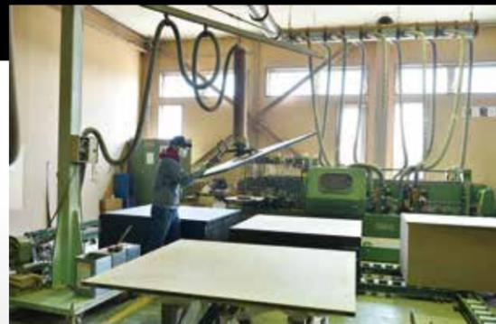
At the finishing area, the table surfaces are inspected one by one after completing the bonding and pressing process.
