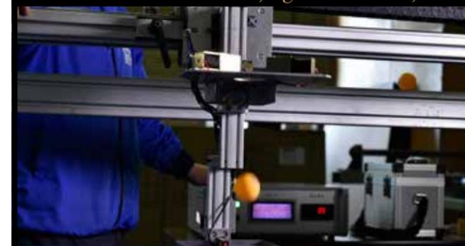
Elements such as bounce, light reflection, and friction are checked against the rigorous guidelines with SAN-EI's proprietary measuring equipment.
