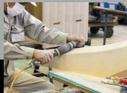
Using a file, the elegant curve of the wooden leg is produced.
