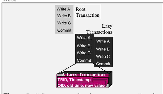
**Figure 4:** A lazy transaction has a root execution that updates either master or local copies of data. Then subsequent transactions update replicas at remote nodes — one lazy transaction per remote replica node. The lazy updates carry timestamps of each original object. If the local object timestamp does not match, the update may be dangerous and some form of reconciliation is needed.
