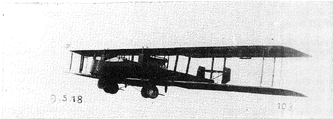
Figure 8: Aircraft with pusher propellers, Fsh-GIIIA The pusher propellers are situated one meter behind the center of gravity.
